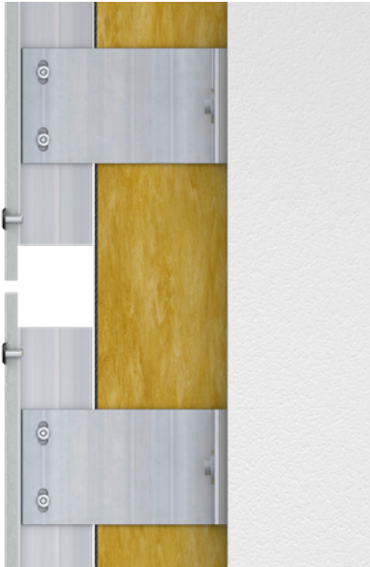
Profile joint = panel joint
