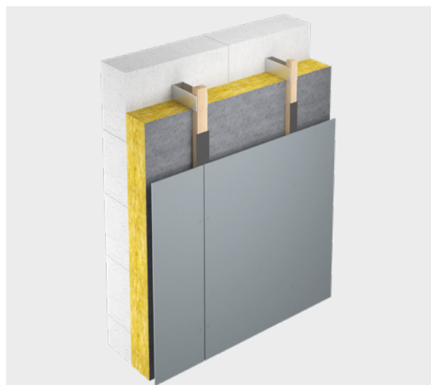
Wooden subframe with spacers
